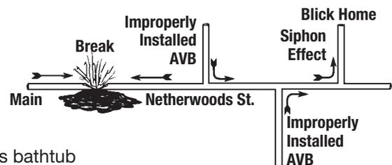
The contractor who installed the sprinkler system didn't pull a city permit and used a "cheap" atmospheric vacuum breaker. When it malfunctioned, which was at the time of the water main break, the nematodes were pulled right in.
